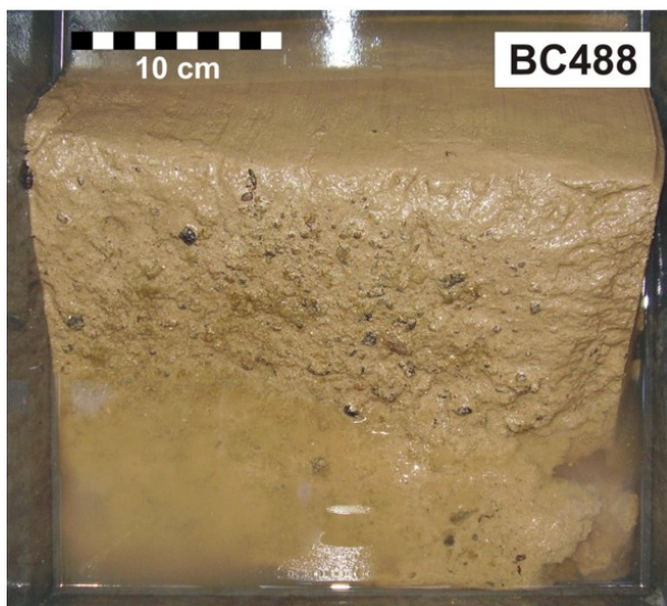
Figure 30: Box core BC488, which apparently fell over during deployment. Note the inclined, but undisturbed sediment surface.
